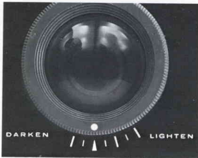
Lighten/Darken control: Set it to the Normal position (shown) unless a label on the back of the film pack (A) shows a special setting. You can open the back of a loaded camera to see if there is such a label. If you do this carefully in the shade or indoors and don't move the pack, the film will not be damaged.
